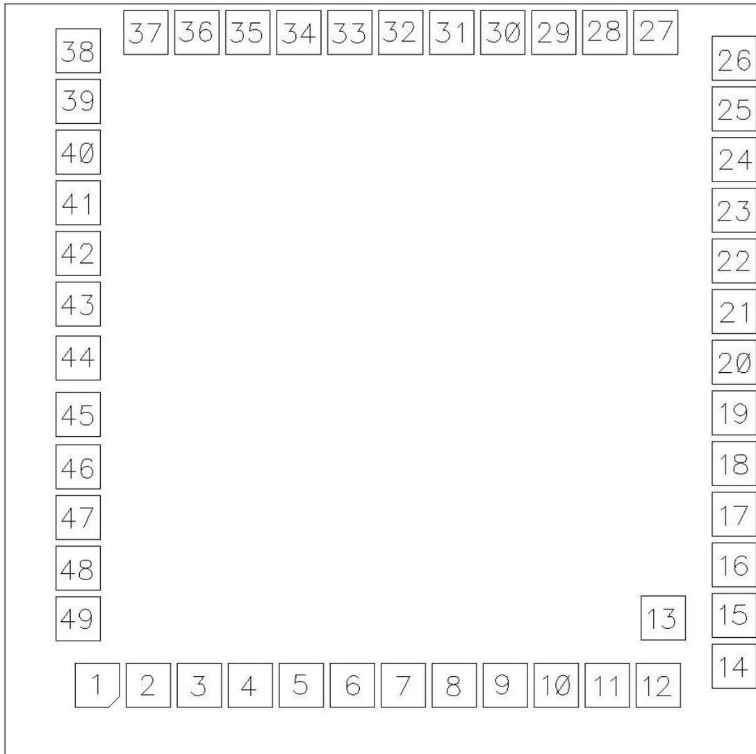
Substrate Size: 1800μm×1800μm
